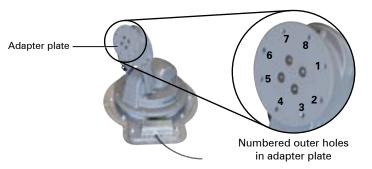
Note: as the antenna raises and turns, the adapter plate may become skewed, and the fourth hole may not be directly at the bottom of the plate. If unsure of the fourth hole, remove the four screws from the center of the adapter plate; a small post is located directly above the fourth hole.
